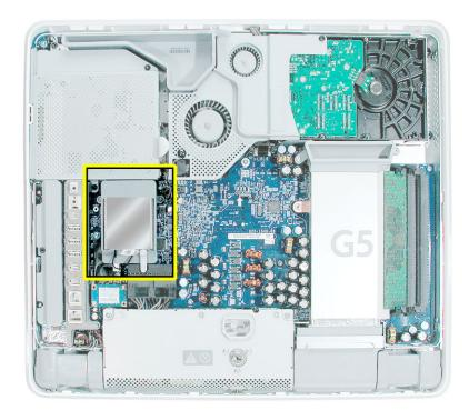
4. Disconnect the antenna cable from the end of the installed AirPort Extreme card.
